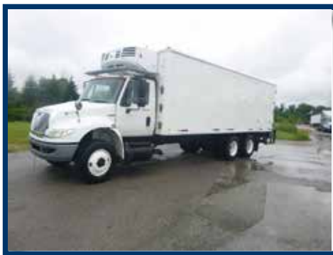
2009 INTERNATIONAL 4400 REEFER BOX TRUCK IHC Maxforce, Allison automatic transmission, 12,000# front axle, 40,000# rears on air ride suspension, 24' Reefer box, Thermo King reefer unit, lift gate, 256" w.b.
