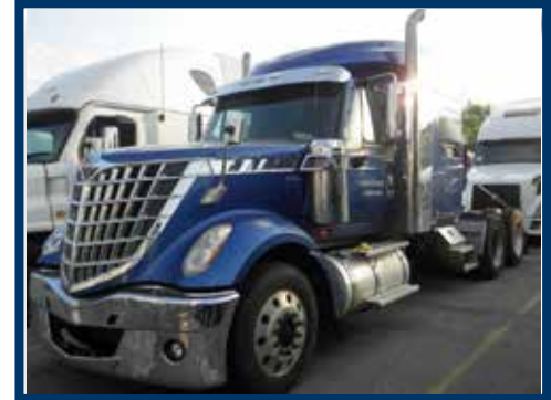
2013 INTERANTIONAL LONESTAR IHC Maxforce w/engine brake, 13 speed transmission, 73" High Rise sleeper cab, 12.350# front axle, 40,000# rears on air ride suspension, air slide 5th wheel, dual high back air ride seats, 242" w.b.
