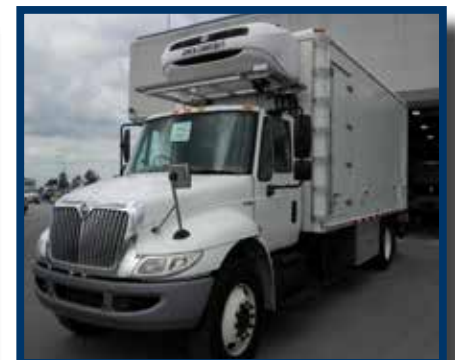
2010 INTERNATIONAL DURASTAR REEFER BOX TRUCK IHC Maxforce, Allison automatic transmission, 12,000# front axle, 21,000# rear axle, spring suspension, 20' reefer box Thermo King reefer unit, swing rear doors, lift gate, tilt/tele, cruise control, 240" w.b.
