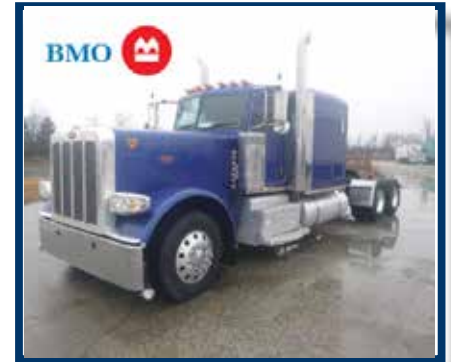
2013 PETERBILT 389 Cummins ISX/525hp w/engine brake, 18 speed transmission, 63" Unibilt Ultracab, 12,000# front axle, 40,000# rears on air ride suspension, air slide 5th wheel, dual high back air ride seats, 11r22.5 rubber on 10 aluminum wheels, 3.42 ratio, heated & power mirrors, tilt/tele, cruise control, 274" w.b.
