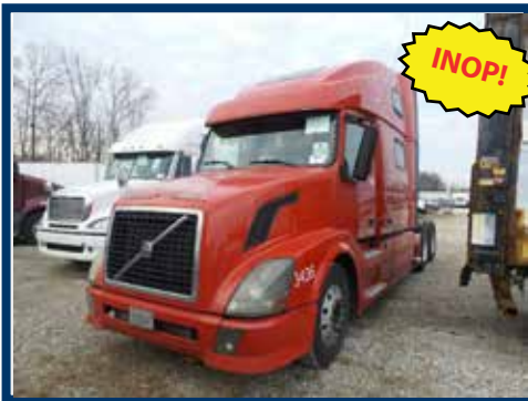
2012 VOLVO VNL64T 780 Cummins ISX/450hp w/ engine brake, 10 speed transmission, 13,200# front axle, 40,000# rears on air ride suspension, air slide 5th wheel, aluminum wheels INOP!!!
