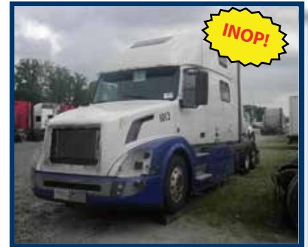
2016 VOLVO VNL64T 780 Volvo VE-D13/500hp w/engine brake, I-Shift transmission, 13,200# front axle, 40,000# rears on air ride suspension, air slide 5th wheel, aluminum wheels, dual 150 gallon fuel tanks INOP!!!
