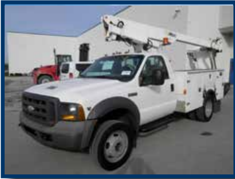
2005 FORD F450 BUCKET TRUCK Ford V10, automatic transmission, 16,000# GVWR, spring suspension, 12' Utility bed, Altec one man bucket, PTO, tilt/tele, cruise control
