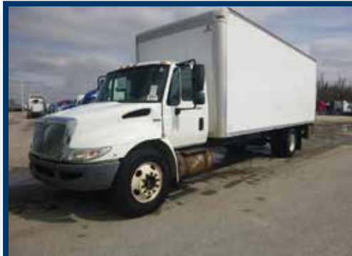
2009 INTERNATIONAL 4300 BOX TRUCK IHC Maxforce, automatic transmission, 25,500# GVWR, spring suspension, 25' box, roll up rear door, lift gate, tilt/tele, cruise control, 256" w.b.
