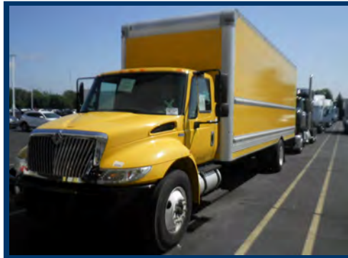
2013 INTERNATIONAL 4300 IHC Maxxforce, automatic transmission, 26' box w/roll-up door, ramp, spring suspension, cruise control, CD player, 272" WB
